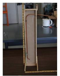
Figure 11 – The one-quarter scale fire model prior to adding insulation.
