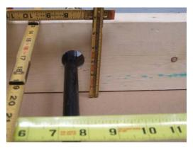
Figure 15 – The enlarged hole where the gas line entered the full-scale fire model wall cavity.
