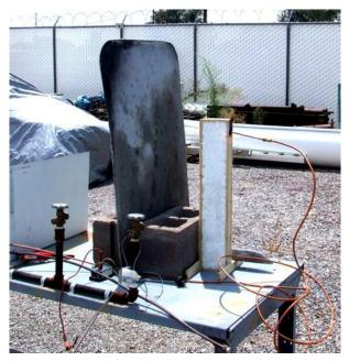
Figure 12 – The one-quarter scale fire model during testing.
