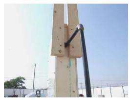
Figure 18 – The location near the top of the full-scale wall cavity where the gas line entered the cavity.
