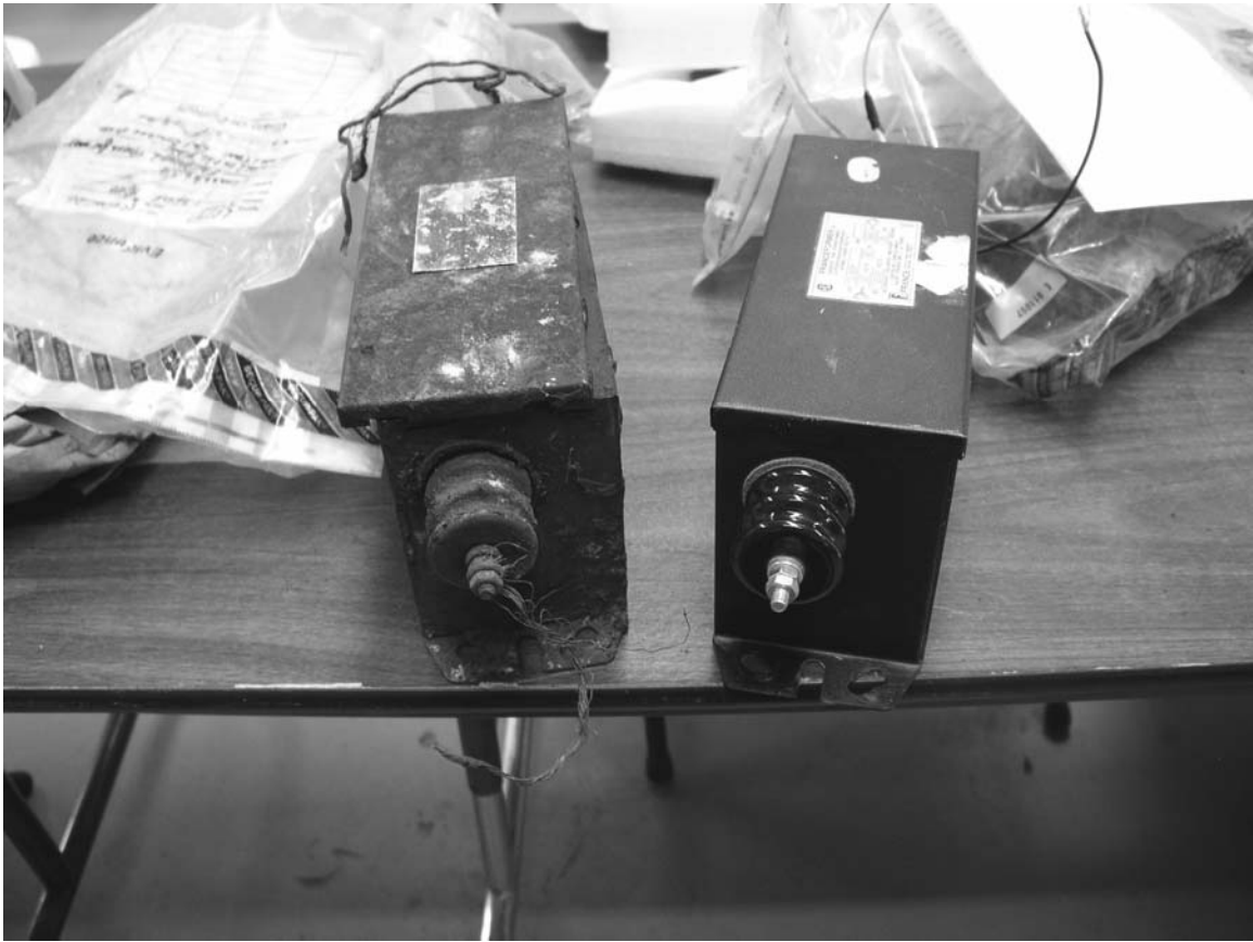
Figure 5 - Recovered and new neon transformers
